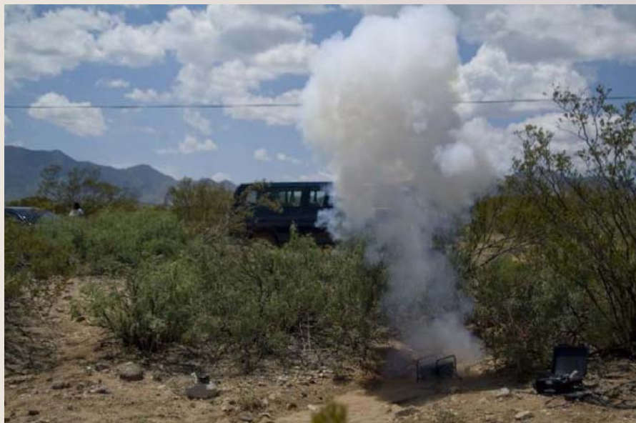
A cold powder charge is set off along a road to demonstrate the new IED simulator. Soldiers and civilians from 19 different installations and facilities came to White Sands Missile Range in New Mexico to learn how to use and maintain the new simulators. (Photo Credit: Drew Hamilton, US Army)
