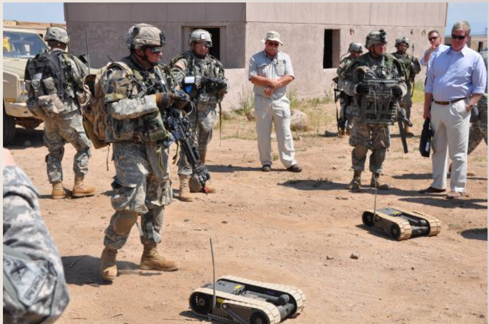
A Soldier from the Army Evaluation Task Force, 5th Brigade, 1st Armored Division, uses a video-game-like controller to steer a Small, Unmanned Ground Vehicle, in the foreground, while another Soldier on his left performs a similar operation with another SUG-V at Adobe Village, White Sands Missile Range, N.M.
