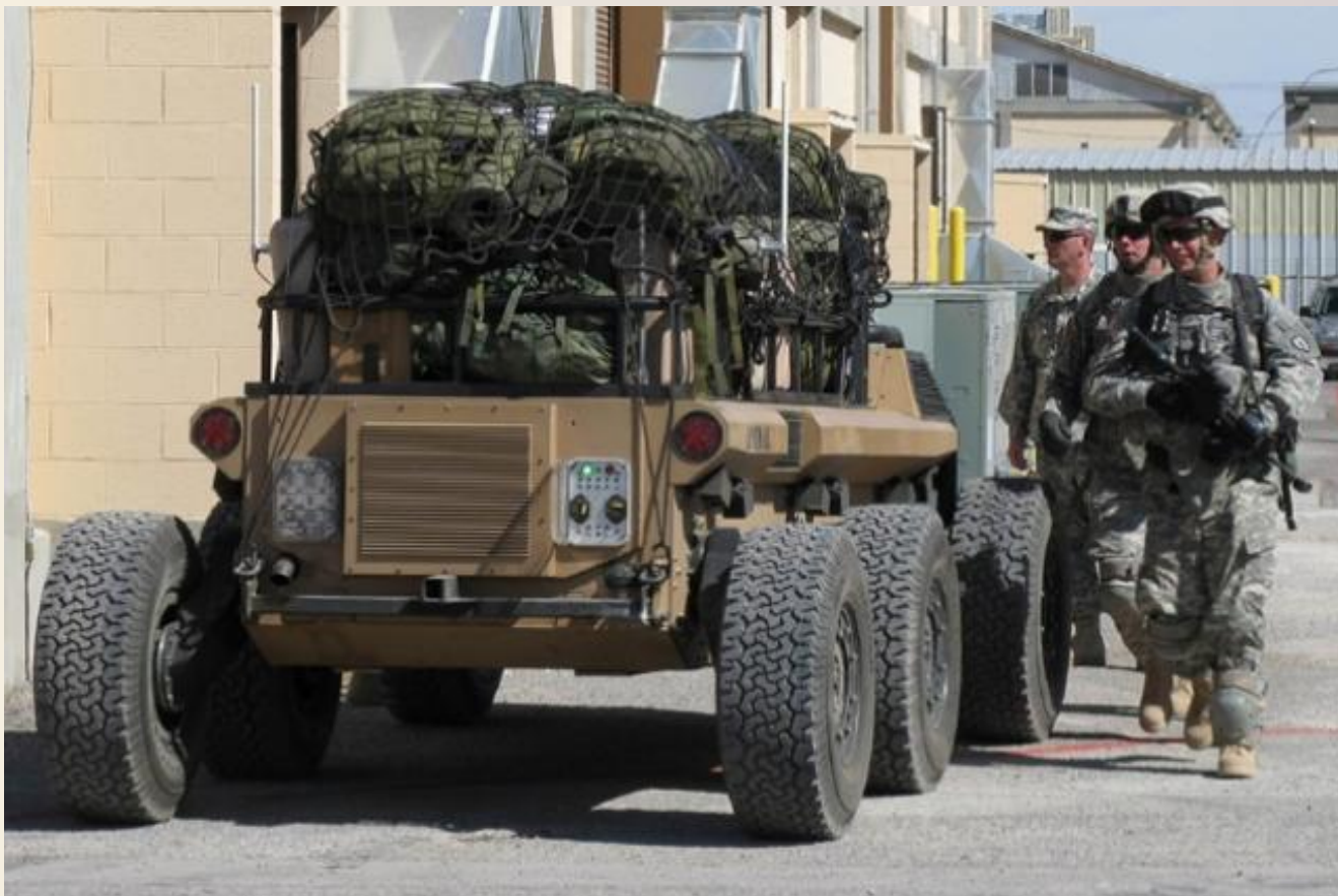
Soldiers of the Army Evaluation Task Force at Fort Bliss test the Multifunctional Utility/Logistics and Equipment vehicle. The MULE is a three-ton unmanned ground system designed to support dismounted, mounted and air assault operations. (Photo Credit: Army)
