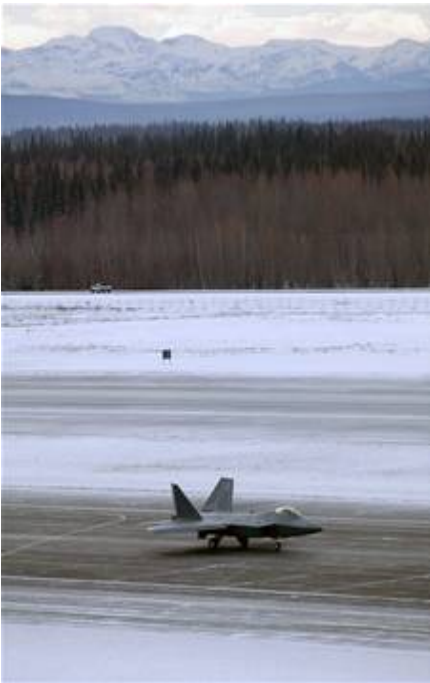
An F-22 Raptor performs 60-knot testing on low runway conditions Nov. 8 at Eielson Air Force Base, Alaska. The F-22 underwent cold-weather testing on its braking system, with emphasis on its ability to maneuver, stop and go on slippery surfaces. The aircraft was tested by the 411th Flight Test Squadron during a three-week deployment on incrementally low-level runway condition reading surfaces, with temperatures ranging between 37 to -13 degrees. The F-22 is from Edwards AFB, Calif. (U.S. Air Force photo/Kevin Roberston)
