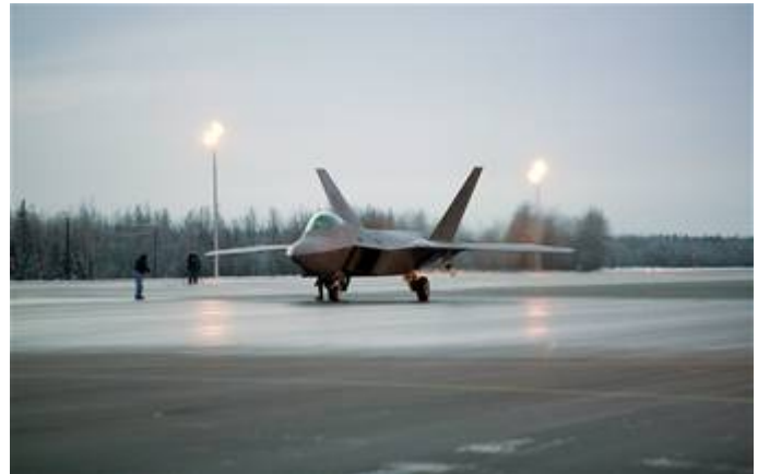
An F-22 Raptor performs maneuvering, stopping and going on low runway conditions Nov. 7 at Eielson Air Force Base, Alaska. The F-22 underwent cold-weather testing on its braking system, with emphasis on its ability to maneuver, stop and go on slippery surfaces. The aircraft was tested by the 411th Flight Test Squadron during a three-week deployment on incrementally low-level runway condition reading surfaces, with temperatures ranging between 37 to -13 degrees. The F-22 is from Edwards AFB, Calif. (U.S. Air Force photo/Kevin Roberston)
