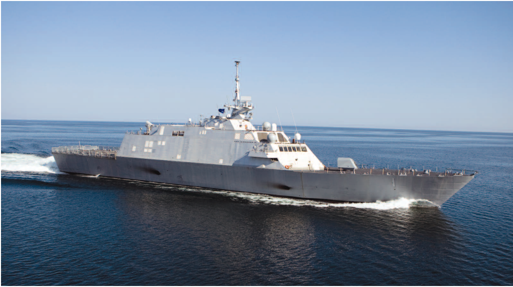
Figure 4. USS Freedom (LCS 1) is the first US Navy Littoral Combat Ship in an entirely new class of Navy surface warships. The ship is designed for littoral, or close-to-shore, operations and to provide access and dominance in coastal-water areas. (Photo provided courtesy of Lockheed Martin)
