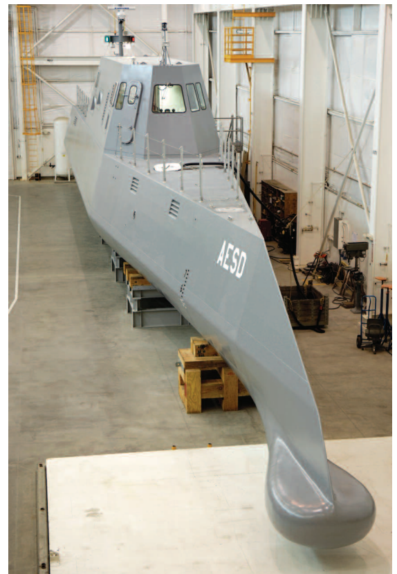
Figure 3. The AESD Sea Jet, funded by the Office of Naval Research, is a 133-foot vessel located at the Naval Surface Warfare Center Carderock Division. (Photos by Mr. John F. Williams and provided courtesy of US Navy)
