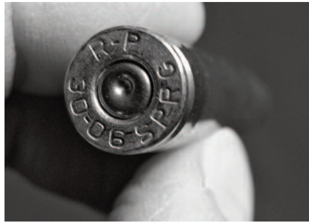
Figure 2. DDNP-based KVB-7E primer which produced a misfire in a 30-06 test load. The crater suggests the misfire was not due to a light primer strike. The other nine 30-06 test loads with this primer demonstrated a perceptible delay in ignition.
